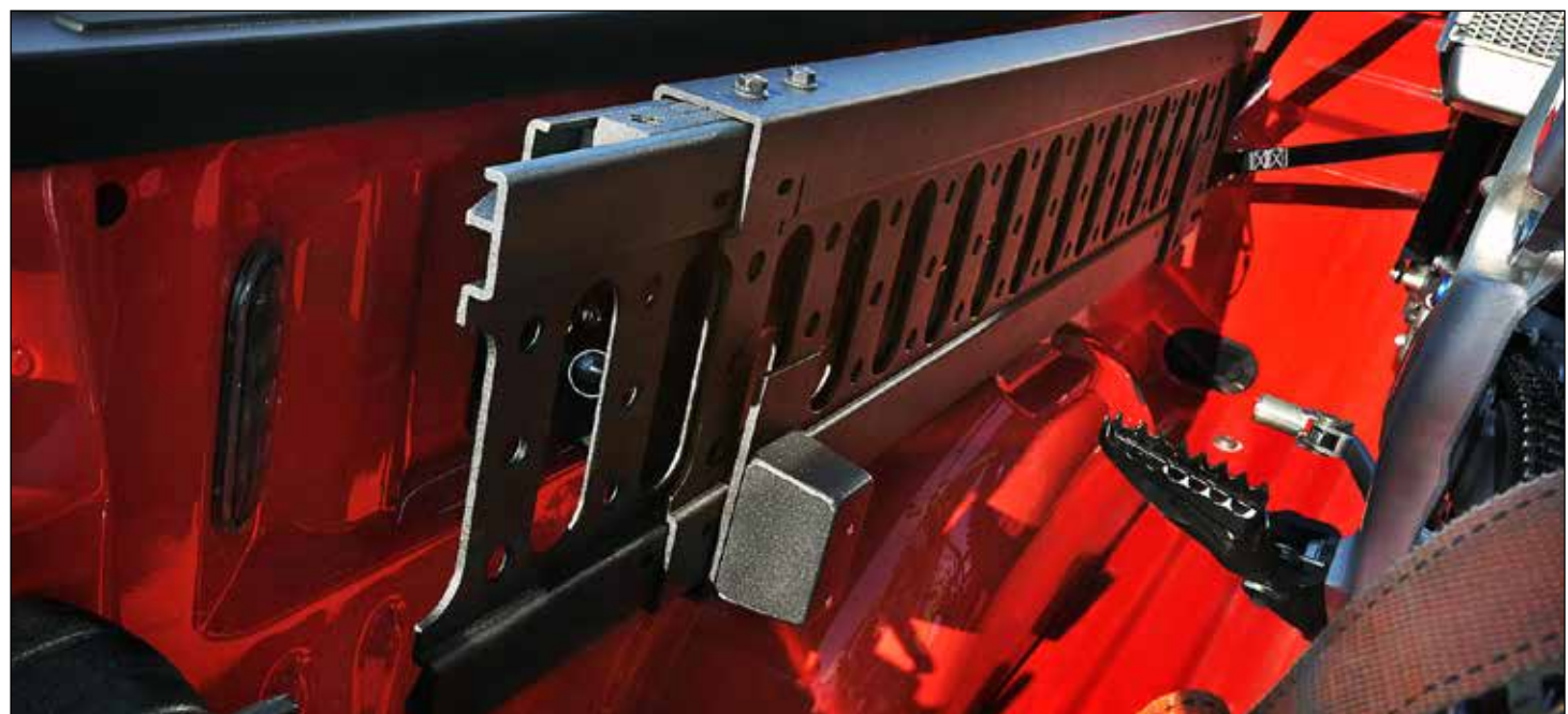
Ford's new BoxLink system offers a wide range of cleats and accessories to secure and store cargo.
