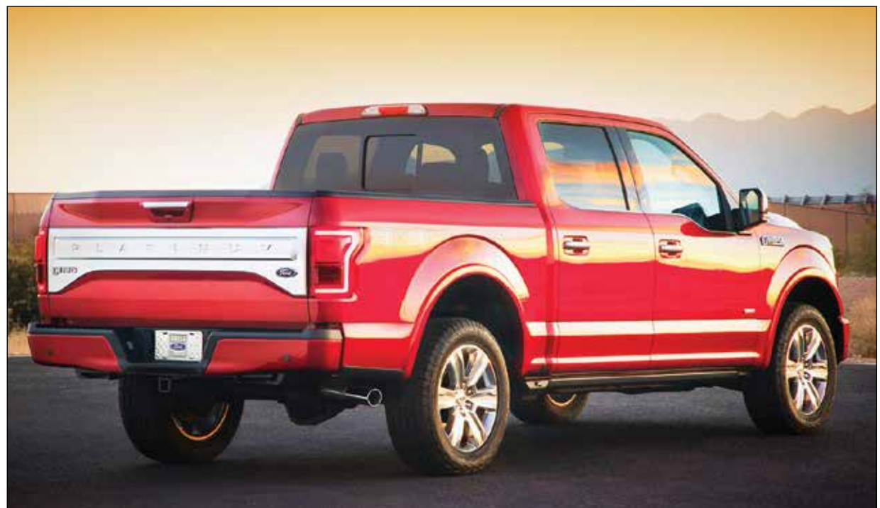
An aluminum body helps the new F-150 shed up to 700 pounds compared to its predecessor, something that improves both performance and fuel economy.
