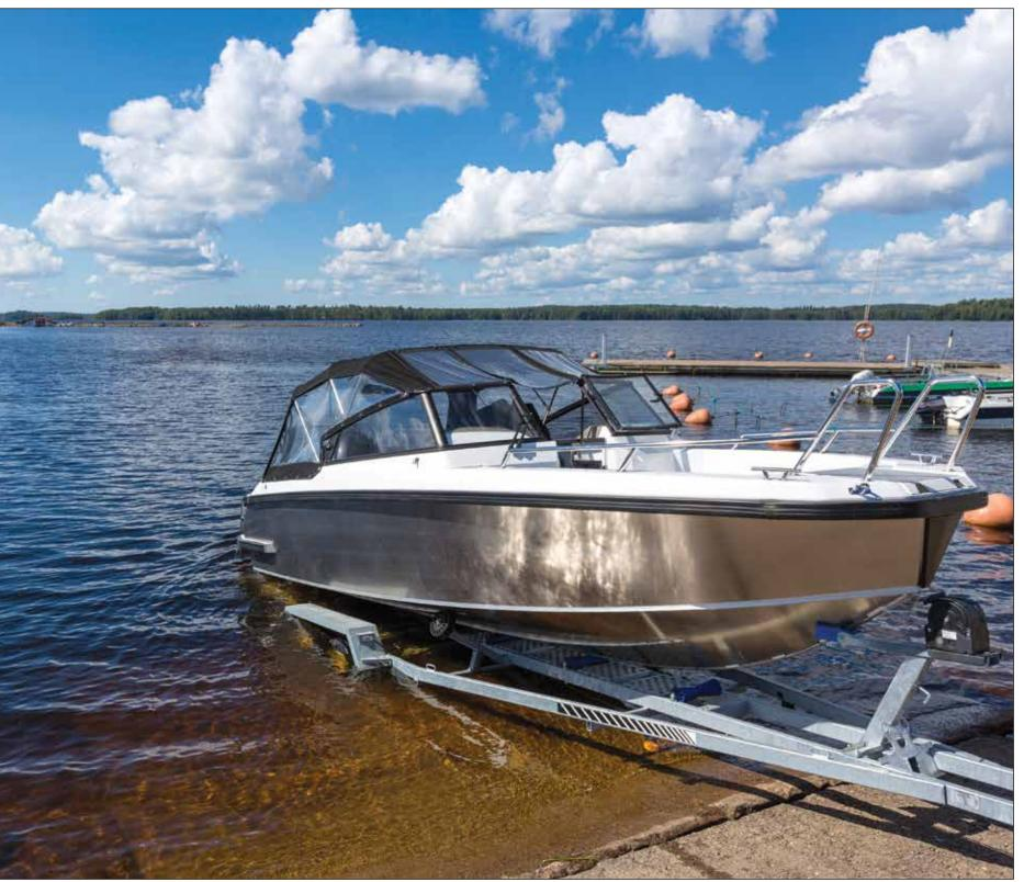
Apply the towing parking brake for your vehicle and, if possible, keep the tires of the actual vehicle away from the water. Slowly release the winch line and reverse your
