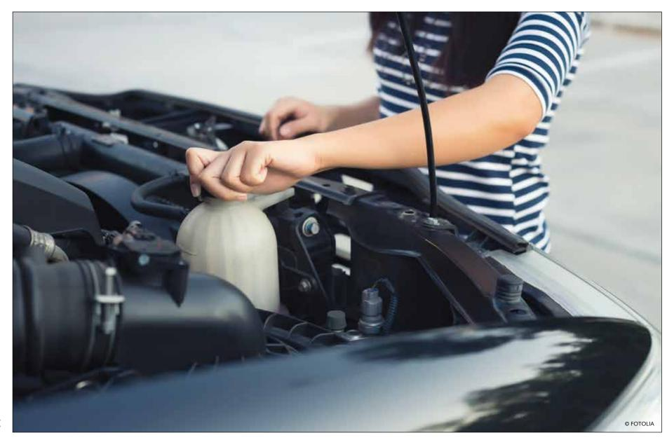
drained and you have allowed the flush to clean up, it is time to close the valve and add the proper amount of antifreeze/ water as noted in your owner's manual. If you don't have an owner's manual, you can easily find this capacity level from a local auto parts store.
